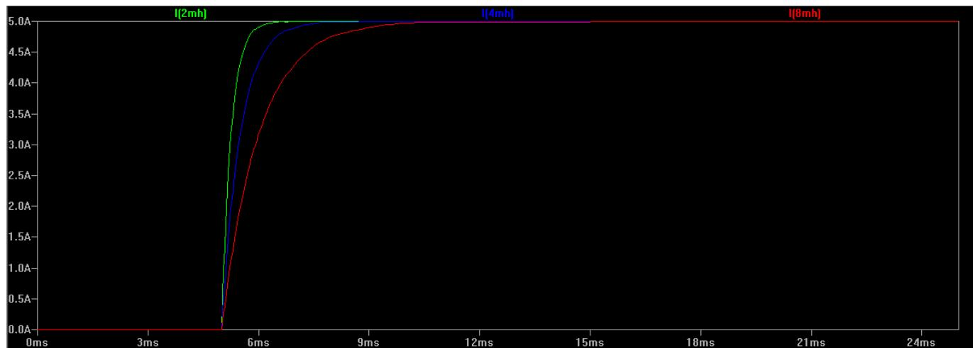
If the rate at which step changes are applied to the coils is significantly shorter than the rise time, it's easy to see that the winding has less time to attain full magnetic attraction on the rotor, and thus maximum torque is curtailed. In the below example the 2 mH coil can achieve the full 5 A limit before the step voltage is removed, but the 4 mH and 8 mH coils cannot:
