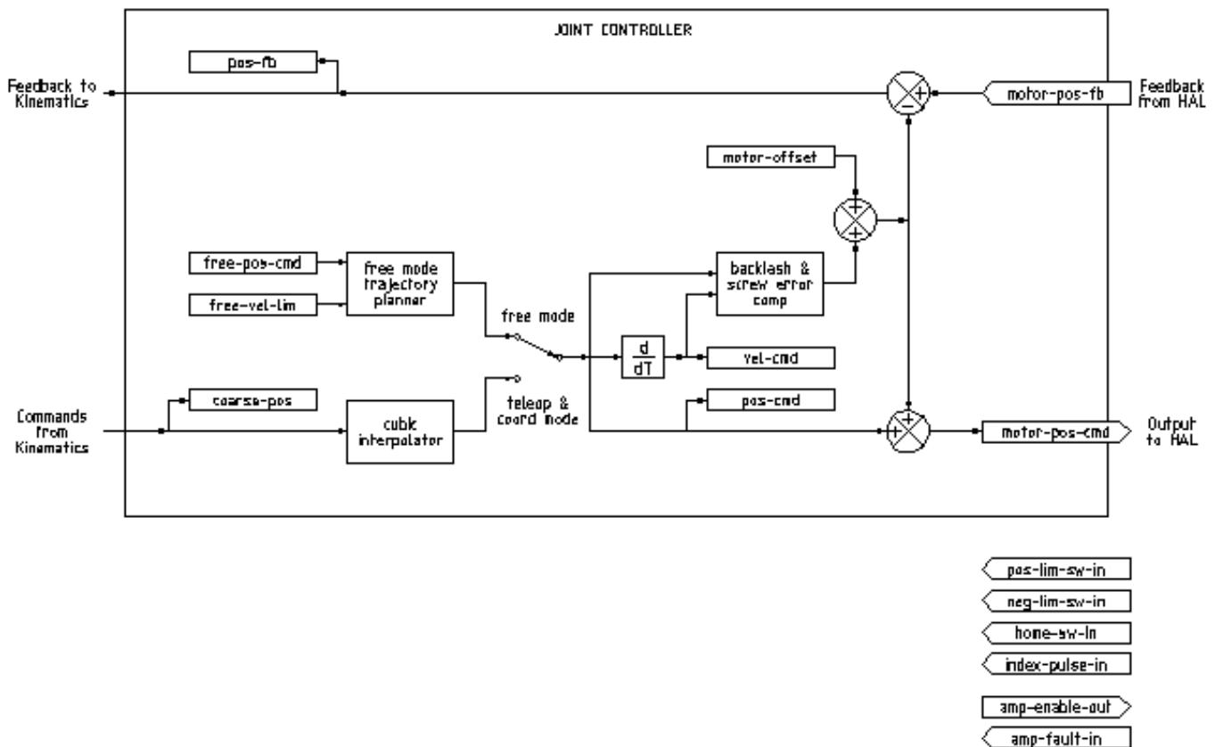
Figure 3.1 – Joint Controller Block Diagram
