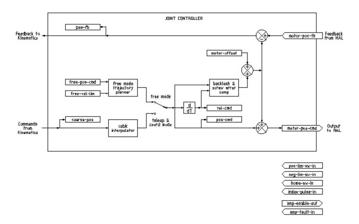
Figur 3.1: Joint Controller Block Diagram
