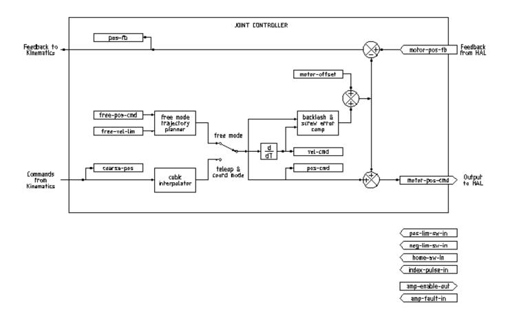
Figure 3.1 - Joint Controller Block Diagram
