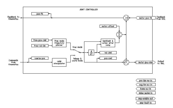
Figure 3.1: Joint Controller Block Diagram
