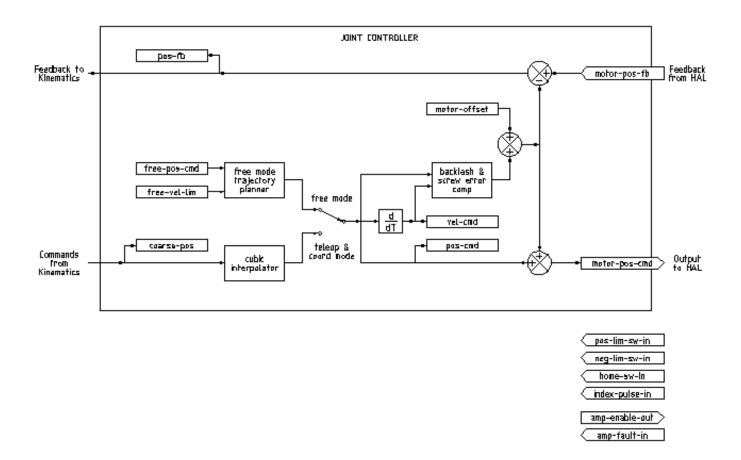
Figur 3.1: Joint Controller Block Diagram
