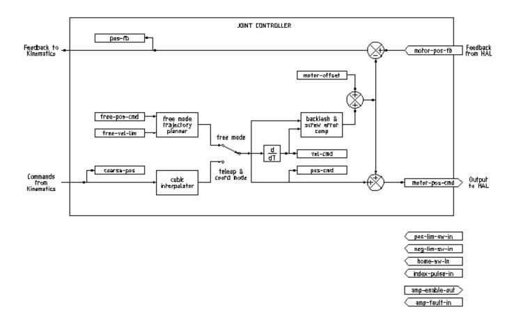
Figure 3.1: Joint Controller Block Diagram
