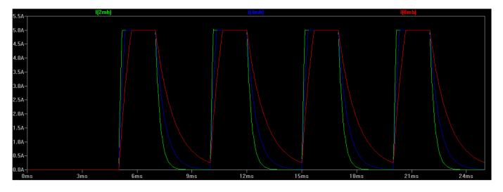
However, careful management of a higher drive voltage is required, as a higher voltage will increase current flowing in each coil with a corresponding increase in temperature of the winding. Excessive temperature rise in the winding will lead to eventual overheating and failure of the motor.
