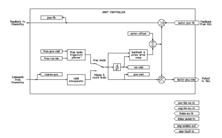
Figure 3.1: Joint Controller Block Diagram
