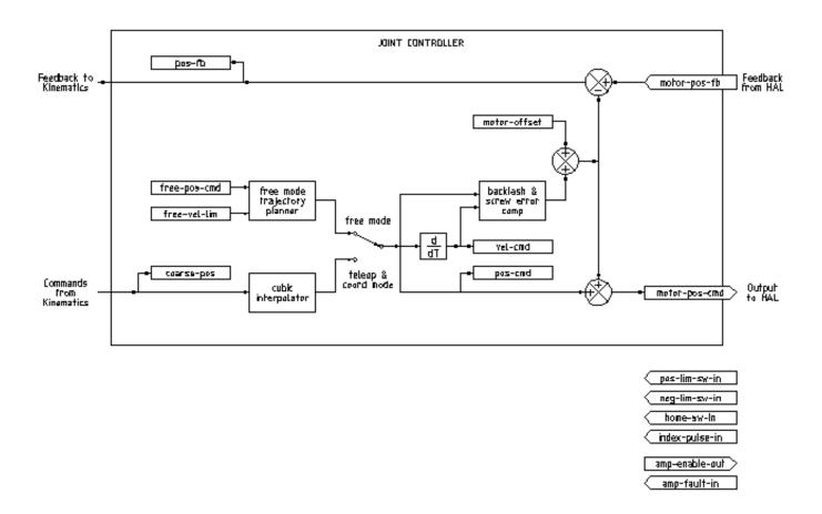
Figure 3.1 - Joint Controller Block Diagram
