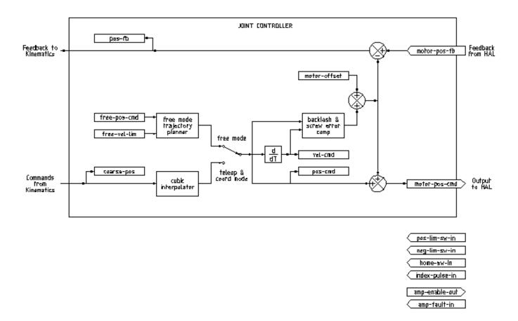
Figur 3.1: Joint Controller Block Diagram
