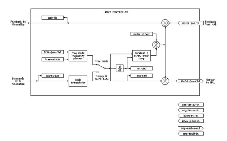
Figure 3.1 - Joint Controller Block Diagram
