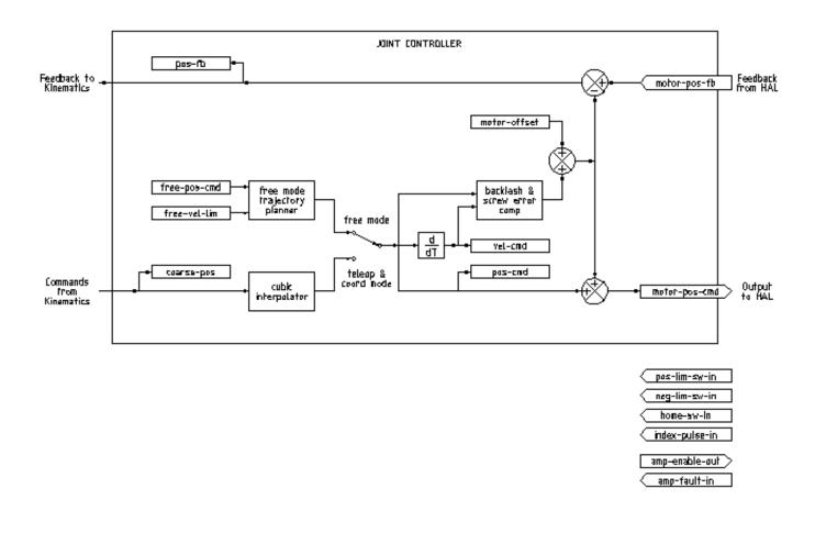
Figure 3.1: Joint Controller Block Diagram
