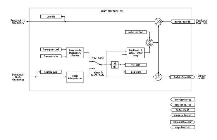
Figure 3.1 - Joint Controller Block Diagram
