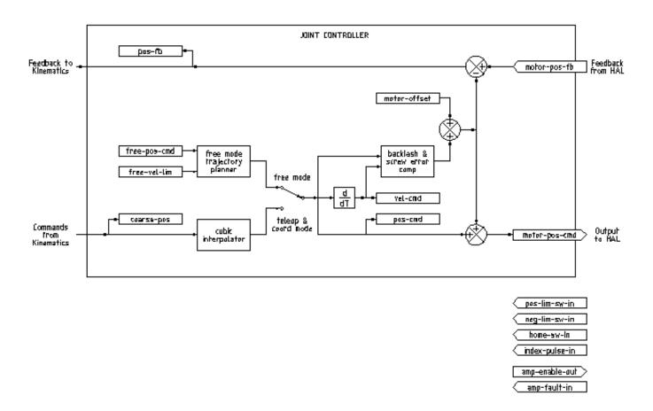
Figur 3.1: Joint Controller Block Diagram
