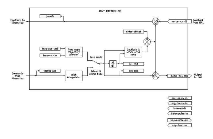
Figura 3.1: Joint Controller Block Diagram
