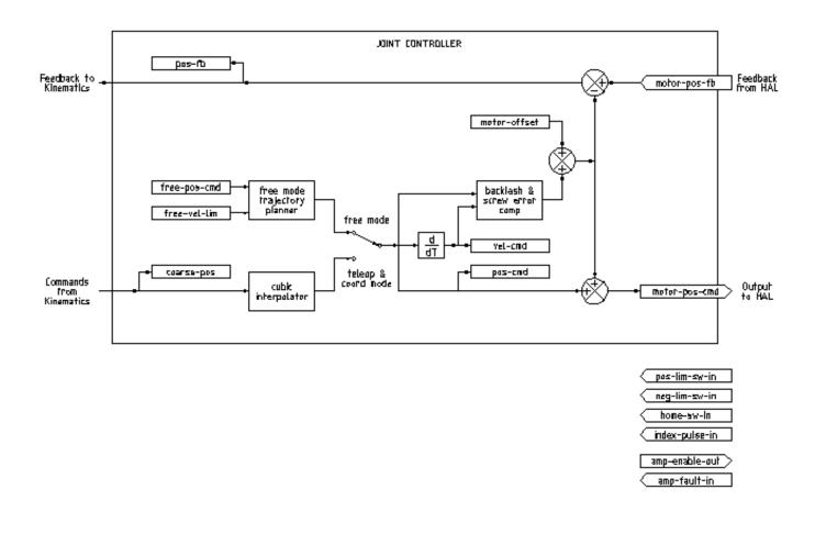
Figure 3.1: Joint Controller Block Diagram
