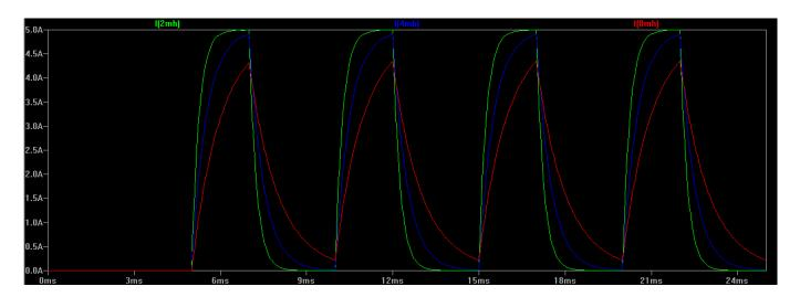
The accepted way of improving motor speed while maintaining torque is to increase the speed at which the magnetic field of the motor coils can expand and collapse. The easiest way to accomplish this is to increase the supply voltage to force the current in each winding to rise and fall much more rapidly. A quicker magnetising time equates to faster step rates while improving torque at higher speeds, both of which are obviously desirable in a CNC system.
