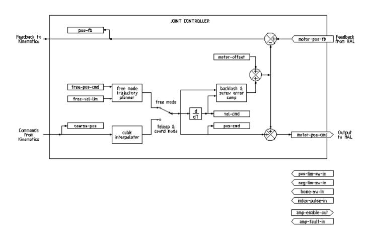
Figure 3.1 - Joint Controller Block Diagram
