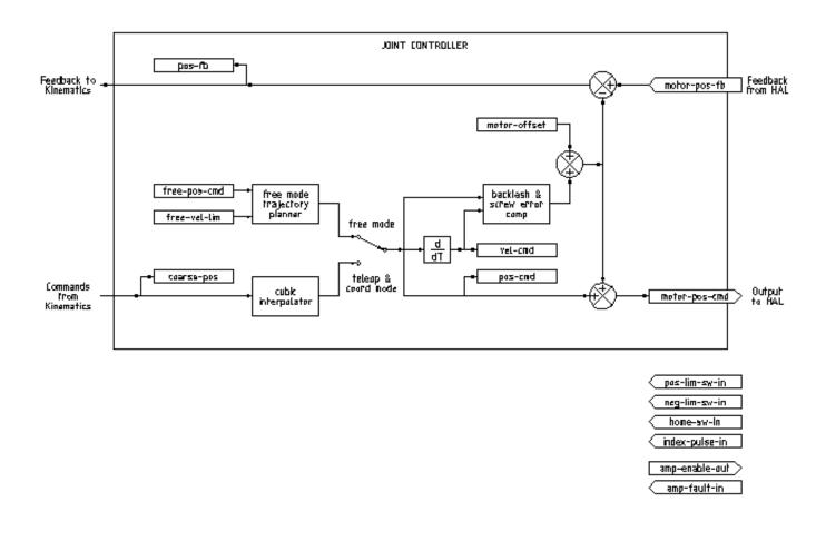
Figur 3.1: Joint Controller Block Diagram
