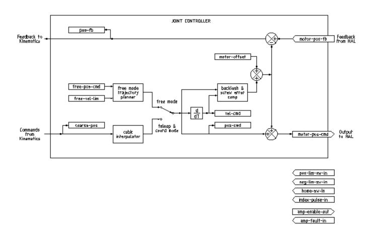
Figure 3.1 - Joint Controller Block Diagram
