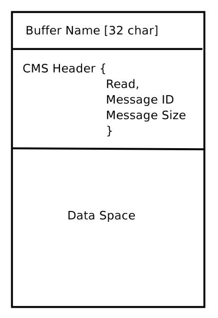
CMS buffer The CMS base class is primarily responsible for creating the communications pathways and interfacing to the operating system.
