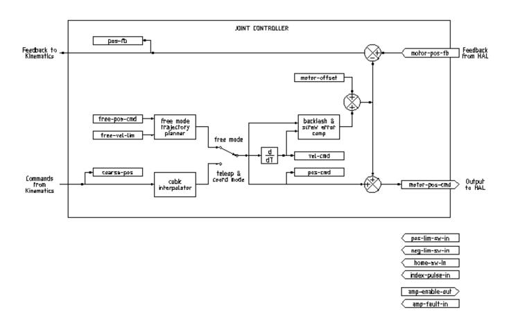
Figure 3.1 - Joint Controller Block Diagram
