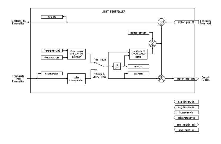
Figura 3.1: Joint Controller Block Diagram
