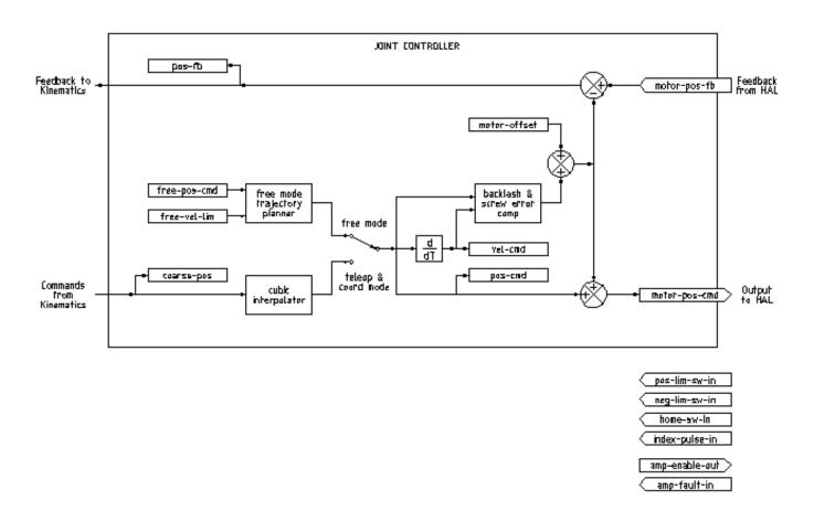
Figure 3.1: Joint Controller Block Diagram
