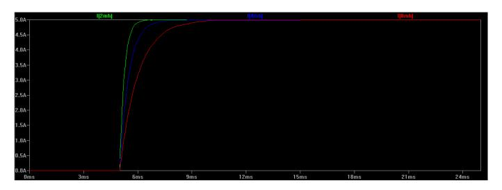
If the rate at which step changes are applied to the coils is significantly shorter than the rise time, it's easy to see that the winding has less time to attain full magnetic attraction on the rotor, and thus maximum torque is curtailed. In the below example the  $2\,\mathrm{mH}$  coil can achieve the full  $5\,\mathrm{A}$  limit before the step voltage is removed, but the  $4\,\mathrm{mH}$  and  $8\,\mathrm{mH}$  coils cannot:
