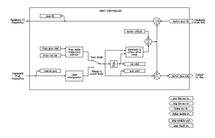
Figure 3.1 - Joint Controller Block Diagram
