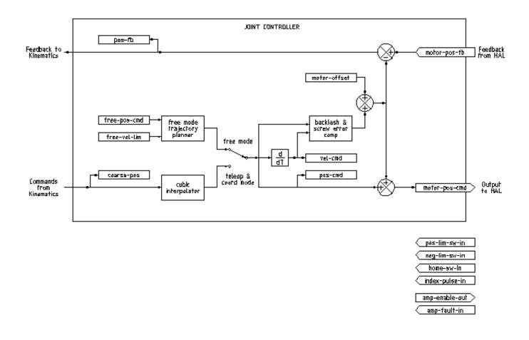
Figure 3.1 - Joint Controller Block Diagram
