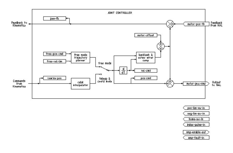
Figure 3.1: Joint Controller Block Diagram
