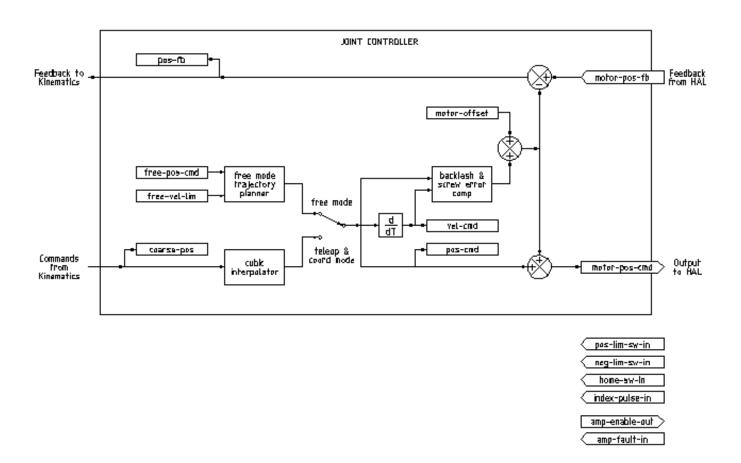
Figure 3.1: Joint Controller Block Diagram
