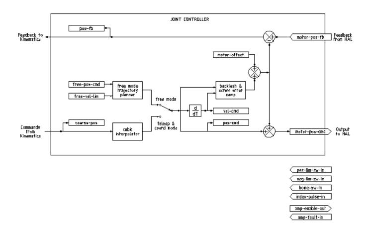
Figure 3.1 - Joint Controller Block Diagram
