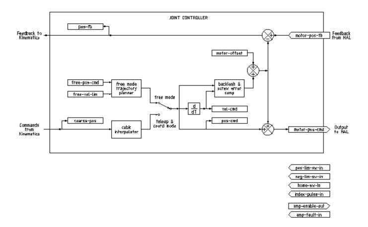
Figure 3.1 - Joint Controller Block Diagram
