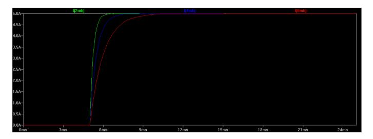
If the rate at which step changes are applied to the coils is significantly shorter than the rise time, it's easy to see that the winding has less time to attain full magnetic attraction on the rotor, and thus maximum torque is curtailed. In the below example the  $2\,\mathrm{mH}$  coil can achieve the full  $5\,\mathrm{A}$  limit before the step voltage is removed, but the  $4\,\mathrm{mH}$  and  $8\,\mathrm{mH}$  coils cannot:
