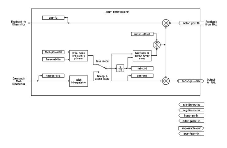
Figura 3.1: Joint Controller Block Diagram
