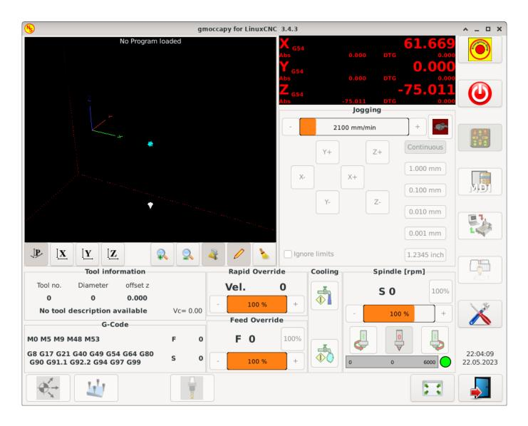
Figure 2.5: GMOCCAPY, a touch screen GUI based on Gscreen
