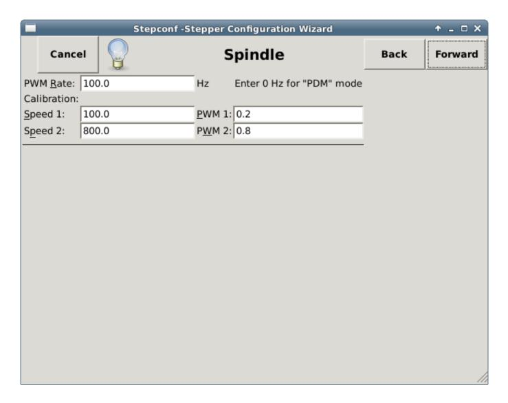
Figure 3.8: Spindle Configuration Page
