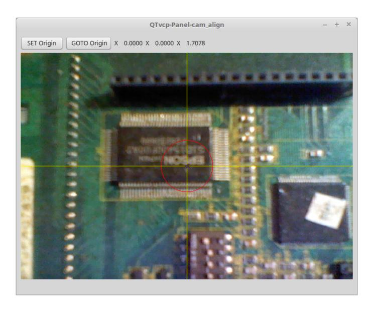
Figure 12.74: QtVCP cam align Panel - Camera Based Alignment Panel
