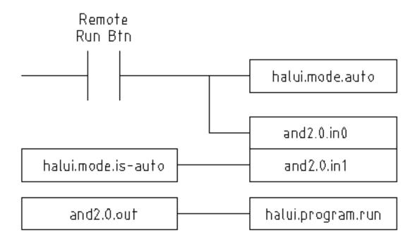
Figure 5.2: Remote Start Example (Schema)
