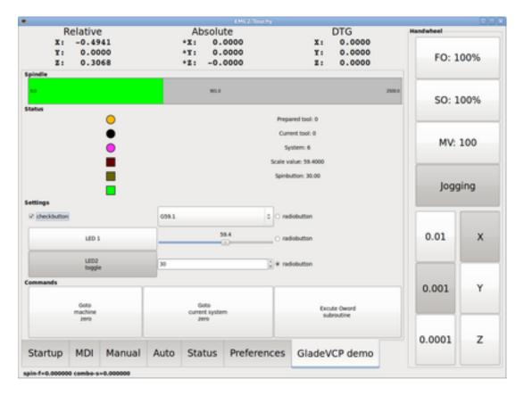
Functionally these setups are identical - they only differ in screen real estate requirements and visibility. Since it is possible to run several GladeVCP components in parallel (with different HAL component names), mixed setups are possible as well - for instance a panel on the right hand side, and one or more tabs for less-frequently used parts of the interface.
