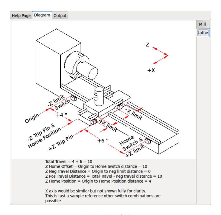
Figure 3.24: AXIS Help Diagram
