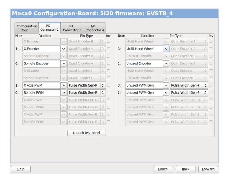
Figure 3.18: Mesa I/O C2 Setup
