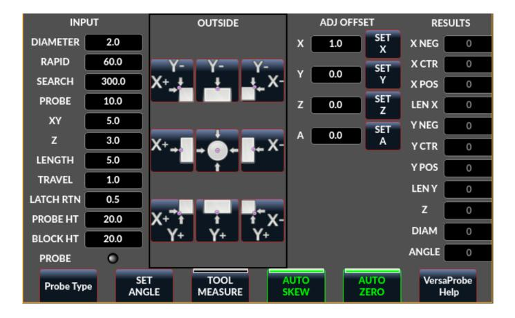
Figure 12.106: QtVCP VersaProbeDialog: Part Touch Probing Dialog Widget
