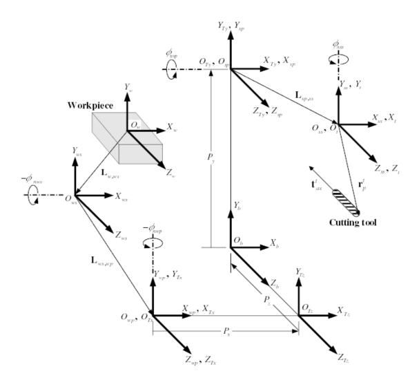
Figure 9.3: General configuration and coordinate systems
