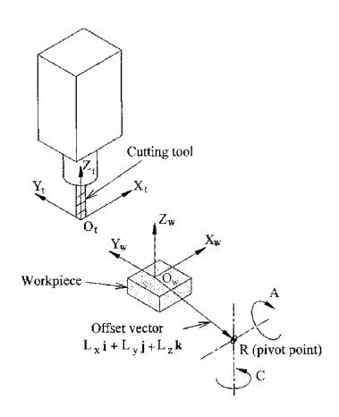
Figure 9.5: Table tilting/rotary configuration
