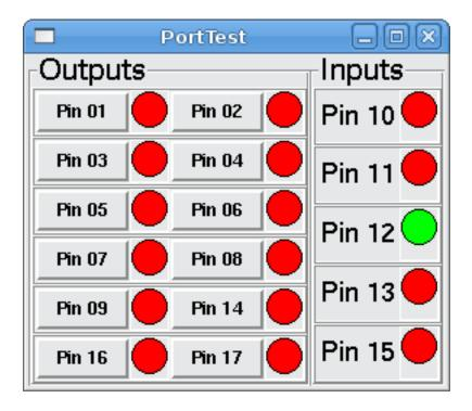
To add the rest of the parallel port pins just modify the XML and HAL files.
