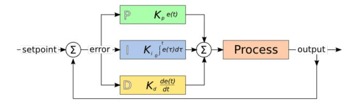
Figure 4.2: PID Loop
