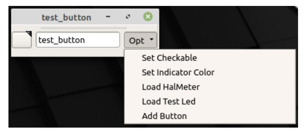
Figure 12.71: QtVCP test button - Test Button VCP
