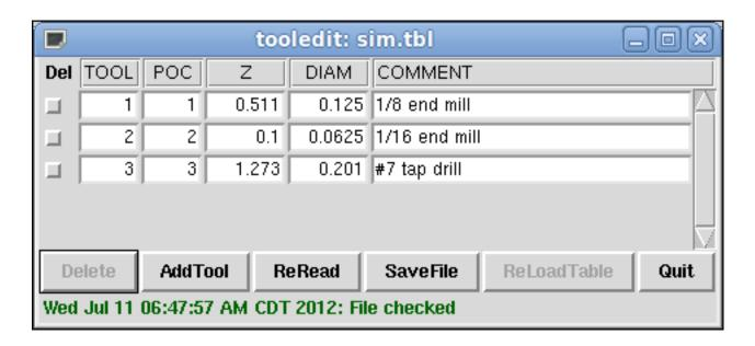
Figure 11.9: Tool Edit GUI - Columns Selection Example
