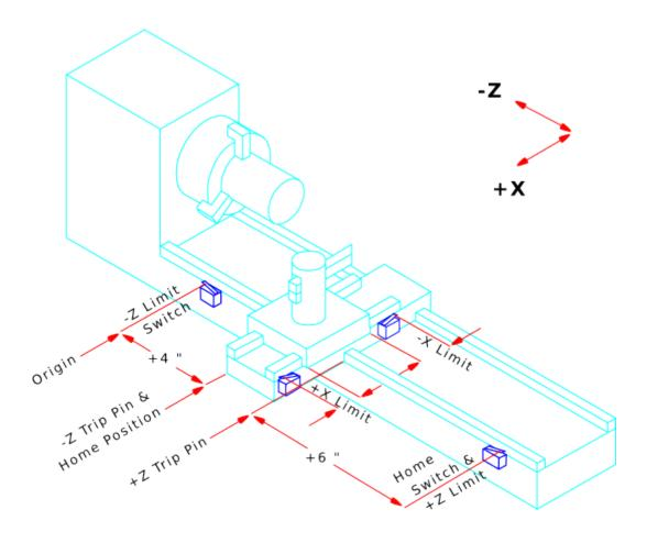
Figure 2.15: Typical Lathe Configuration
