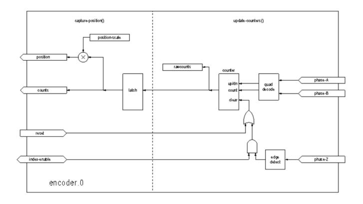
Figure 5.24: Encoder Counter Block Diagram
