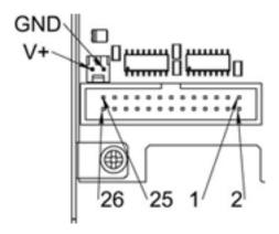
Figure 6.7: Pin numbering of homing & end switch connector
