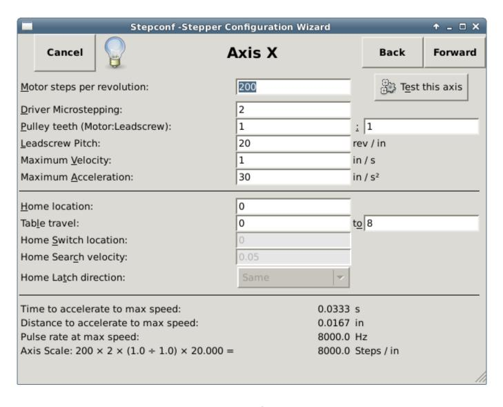
Figure 3.6: Axis Configuration Screen
