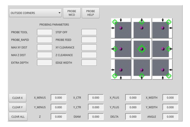
Figure 12.88: QtVCP BasicProbe: Simple Mill Probing Widget
