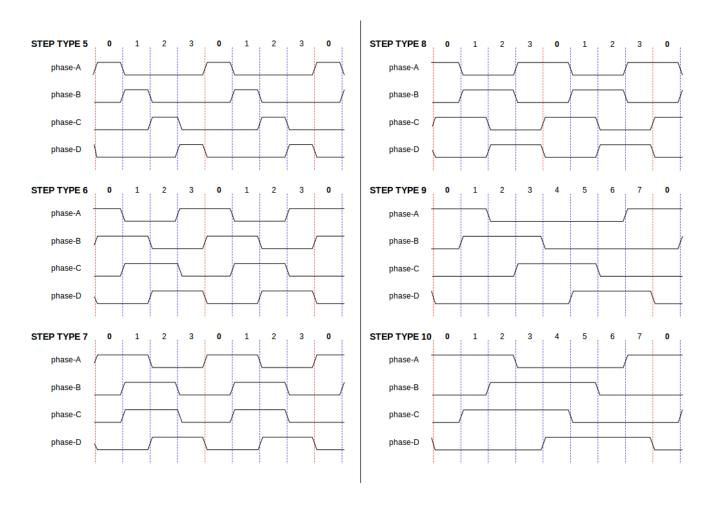
Figure 5.22: Four-Phase Step Types
