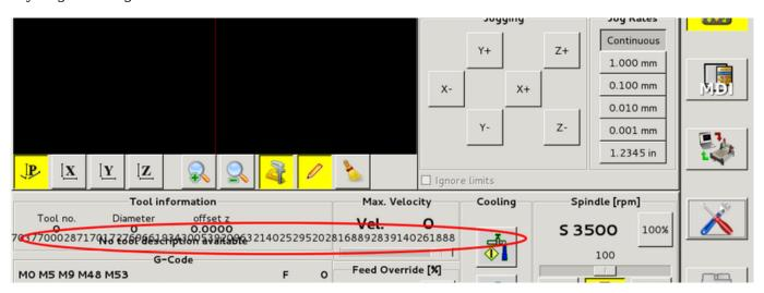
You have made your config file using an older version of StepConfWizard. It has made a wrong entry in the INI file under the [TRAJ] named MAX\_LINEAR\_VELOCITY = xxx. Change that entry to MAX\_VELOCITY = xxx.
