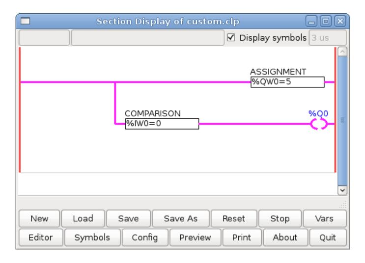
Figure 8.8: Assign/Compare Ladder Example
