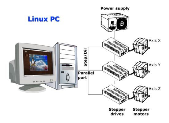
Figure 2.1: Simple LinuxCNC Controlled Machine
