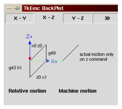
With this program, in most cases, the machine will apply the offset in the form of a ramp during the movement in xyz following the word G43.
