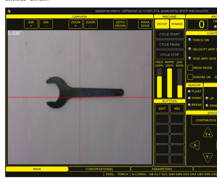
QtPlasmaC has the ability to use a USB camera to set the origin with or without rotation compensation. Rotation compensation can be used to align the work offset to a sheet of material with edge(s) that are not parallel to the machine's X/Y axes. The CAMERA button will be enabled after the machine is homed.
