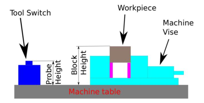
Figure 10.32: Auto tool measurement
