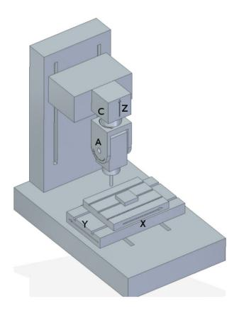
Figure 9.12: Spindle tilting/rotary configuration
