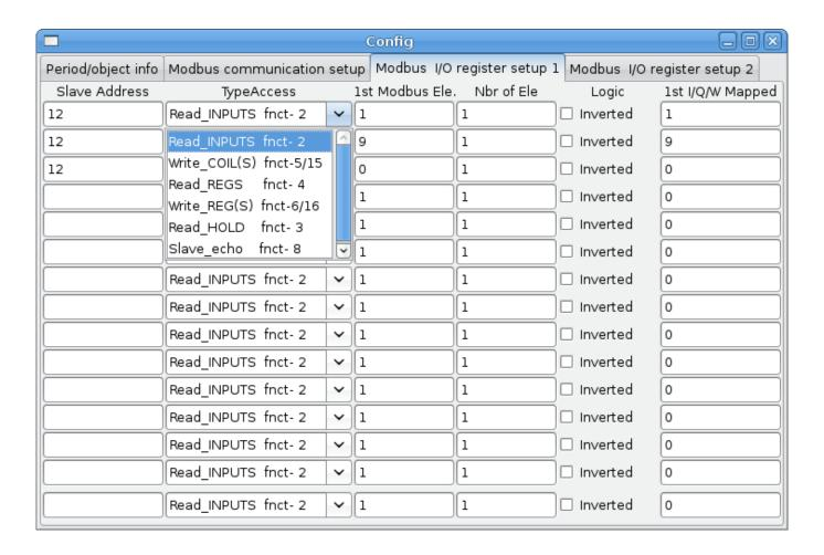
Figure 8.12: Modbus I/O Config
