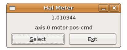
Figure 5.28: Halmeter watch window
