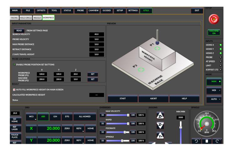
Figure 10.33: QtDragon hd - Work piece Height probing
