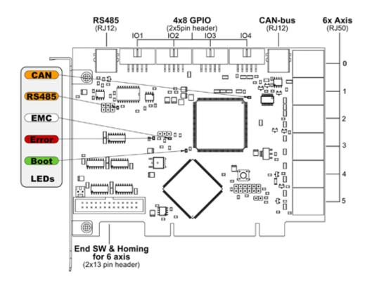
Figure 6.2: GM6-PCI card connectors and LEDs
