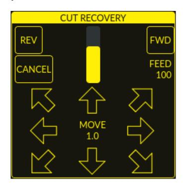
This feature will produce a CUT RECOVERY panel that will allow the torch to be moved away from the cut path during a paused motion event in order to position the torch over a scrap portion of the material being cut so that the cut restarts with a minimized arc-divot. The CUT RECOVERY panel will display automatically over top of the JOGGING panel when motion is paused.
