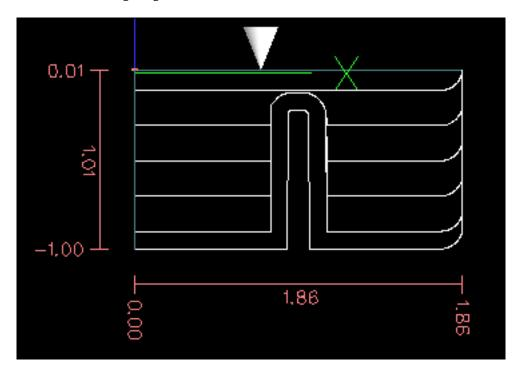
Figure 11.17: Roughing passes and final pass
