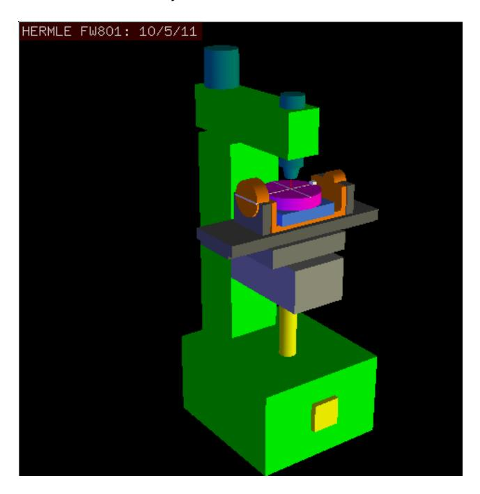
Figure 9.4: vismach model of xyzac-trt with coincident rotation axes
