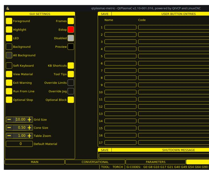
This tab is used to display GUI configuration parameters, button text, and shutdown text that are modified infrequently as well as some utility buttons.
