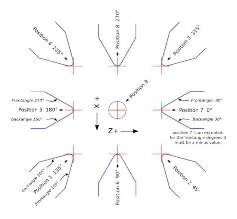
Figure 2.16: Lathe Tool Orientations
