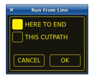
**HERE TO END** will run from the beginning of the selected line to the end of the G-code file with the option of adding a leadin.
