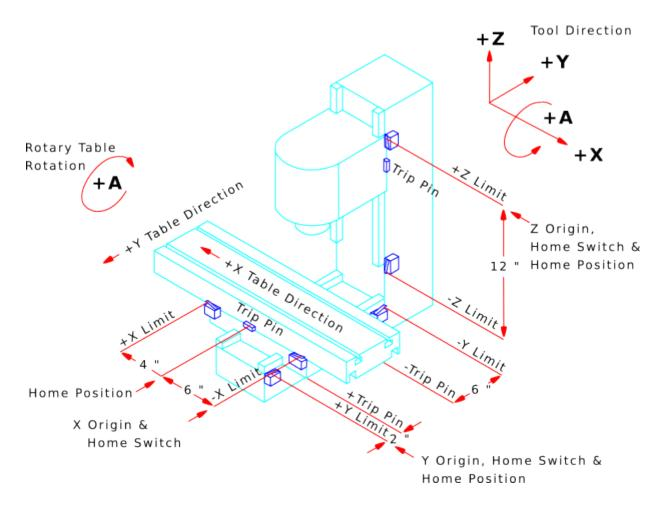
Figure 2.14: Typical Mill Configuration
