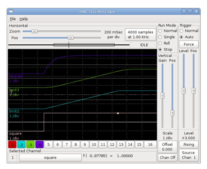
To see the effect of changing the set point values of any of the components you can change them in the terminal window. To see what different gain settings do for lowpass just type the following in the terminal window and try different settings.
