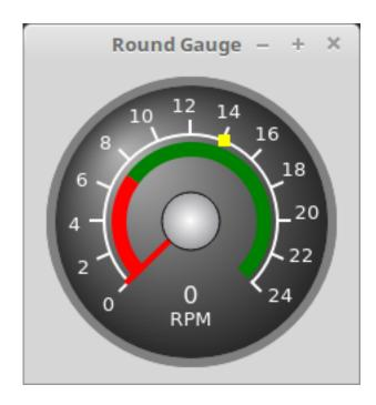
Figure 12.84: QtVCP Gauge: Round Dial Gauge Widget
