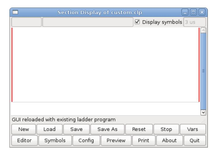
Figure 8.2: Section Display Default Window
