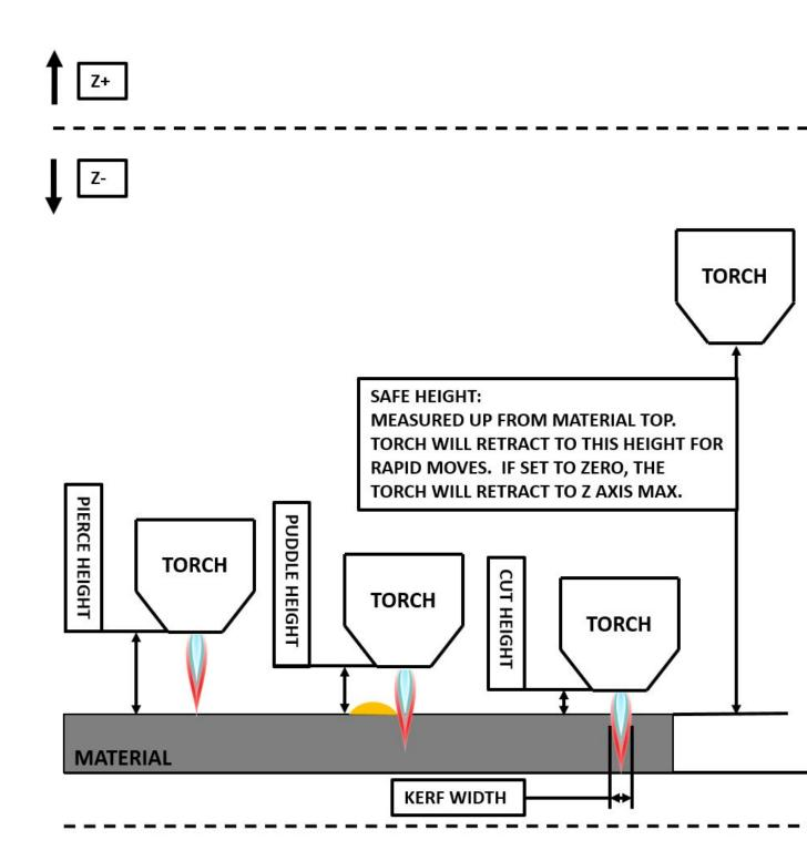
Click on the Parameters Tab to view the **CONFIGURATION** section which shows the user settable parameters. It is necessary to ensure every one of these settings is tailored to the machine.
