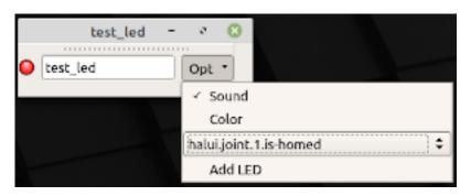
Figure 12.72: QtVCP test\_dial Panel - Test LED VCP
