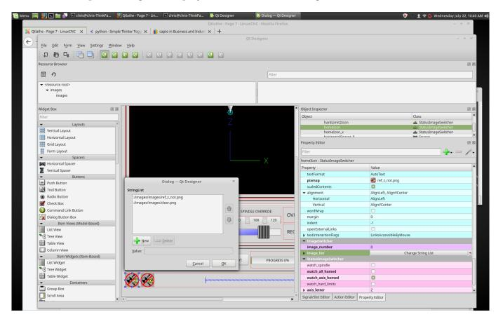
Figure 12.94: QtVCP StatusImageSwitcher: Controller Status Image Switcher
