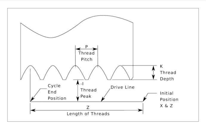
Figure 11.14: G76 Threading
