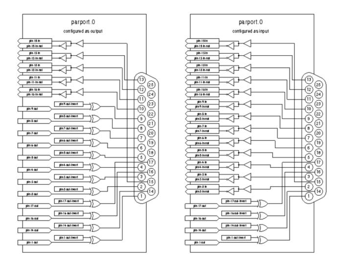
Figure 6.1: Parport block diagram
