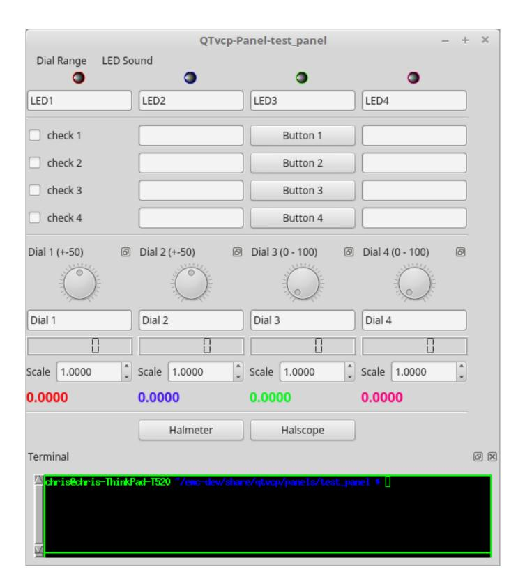
Figure 12.73: QtVCP test\_panel - HAL Component Testing Panel
