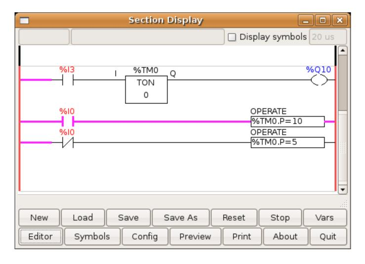
Figure 8.27: Timer/Operate Example
