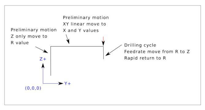
**Example 4 - Absolute G81 R > Z** This is a plot of the path of motion for the second g81 block of code.
