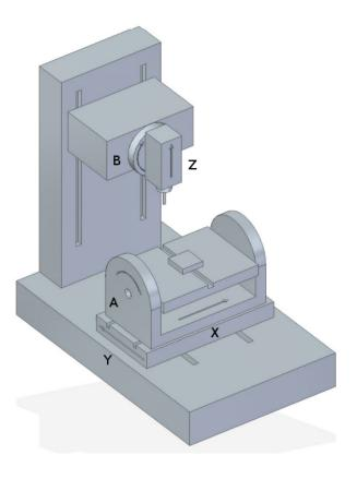
Figure 9.11: Spindle/table tilting configuration
