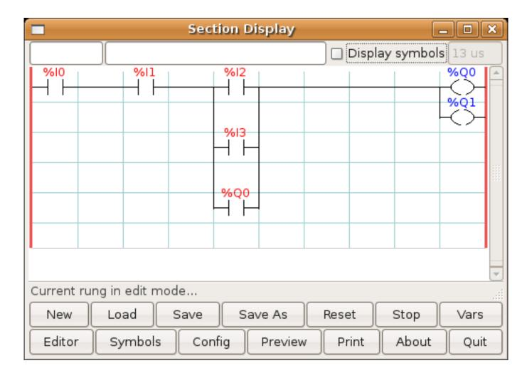
Figure 8.25: E-Stop Section Display
