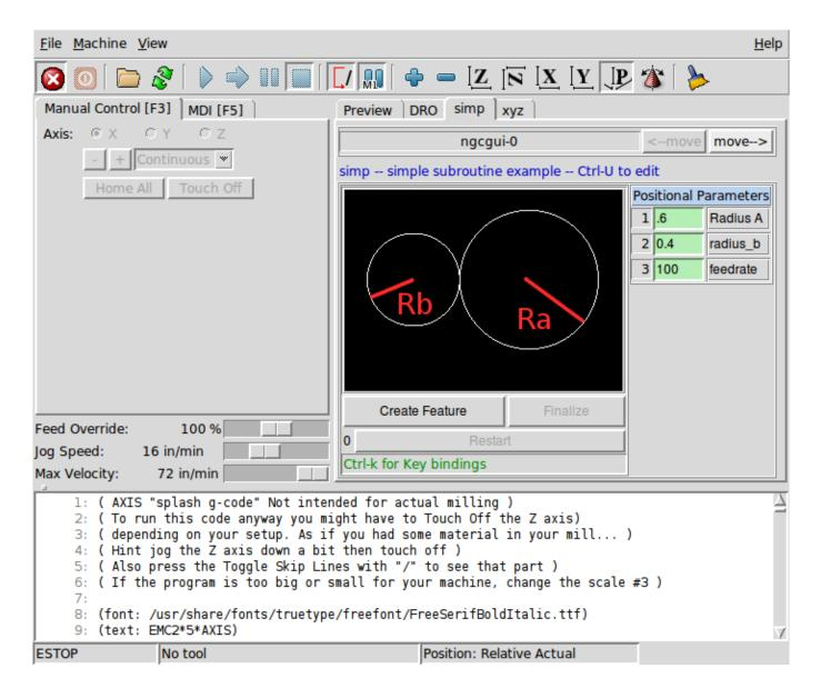
Figure 10.37: NGCGUI embedded into AXIS
