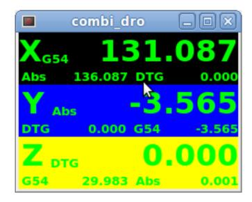
Figure 12.45: Example: Three Combi DRO in a window
