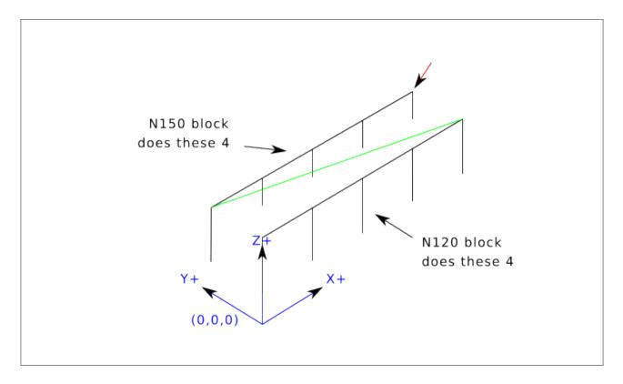
**Twelve Holes in a Square** This example demonstrates the use of the L word to repeat a set of incremental drill cycles for successive blocks of code within the same G81 motion mode. Here we produce 12 holes using five lines of code in the canned motion mode.
