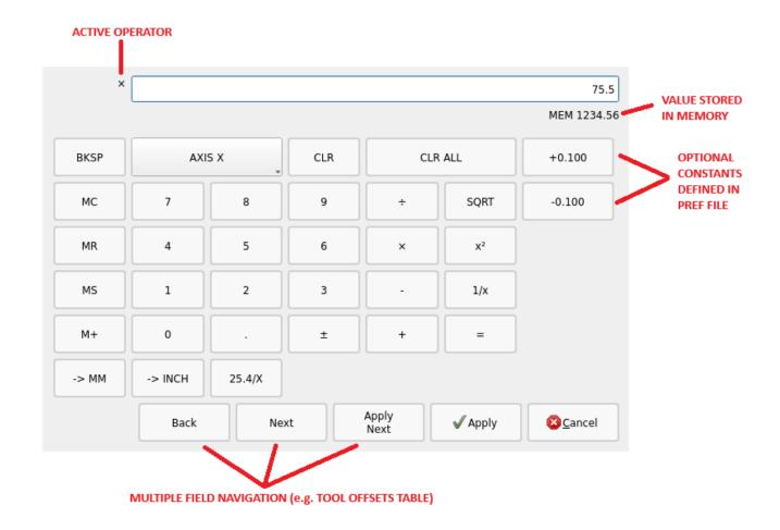
Figure 12.104: QtVCP CalculatorDialog: Calculator Dialog Widget
