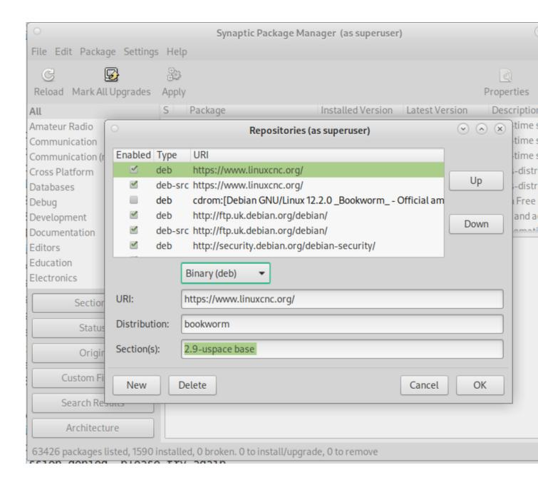
Figure 1.2: Figure with a screenshot of the repository configuration of the synaptic package manager.
