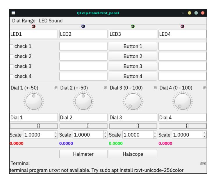
Figure 12.62: QtVCP HAL Test Builtin Panel
