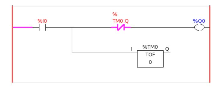
Figure 8.24: Reject Extra Pulse
