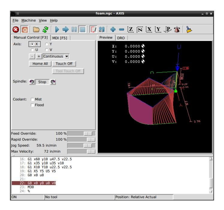
Figure 10.12: Foam Cutting Mode
