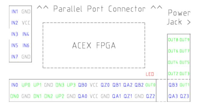
Figure 6.10: Pluto-Servo Pinout
