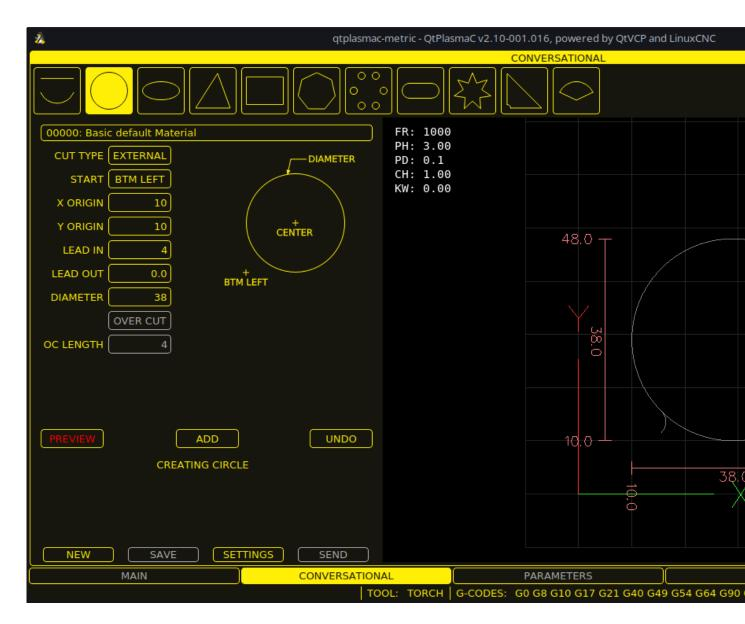
The CONVERSATIONAL Tab enables the user to quickly program various simple shapes for quick cutting without the need for CAM software.
