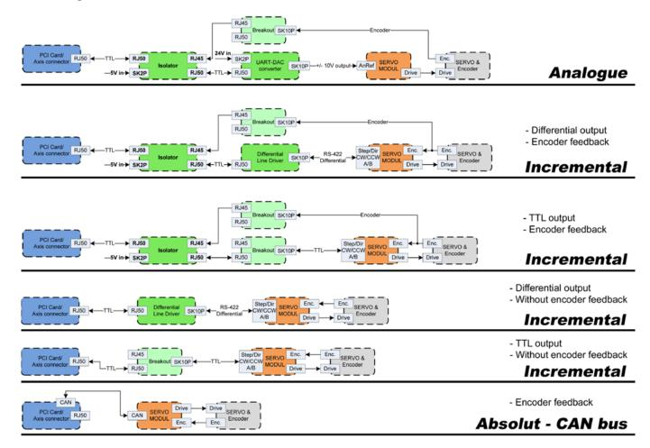
Figure 6.5: Servo axis interfaces
