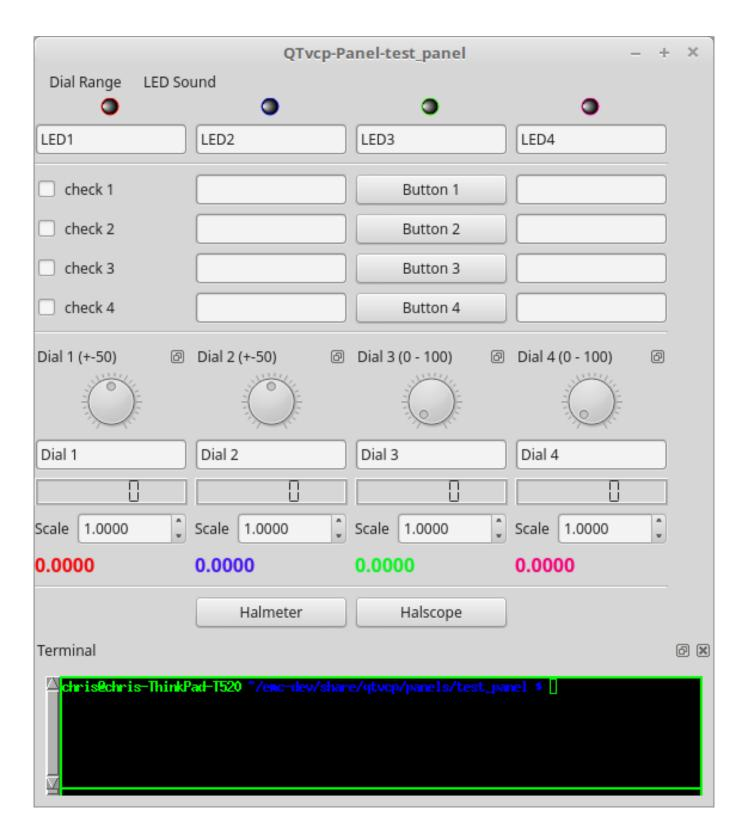
Figure 12.61: test\_panel - Test Panel VCP
