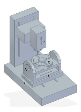
Figure 9.10: Table tilting/rotating configuration
