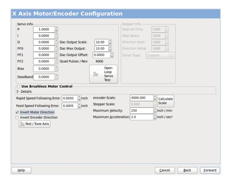
Figure 3.21: Axis Drive Configuration
