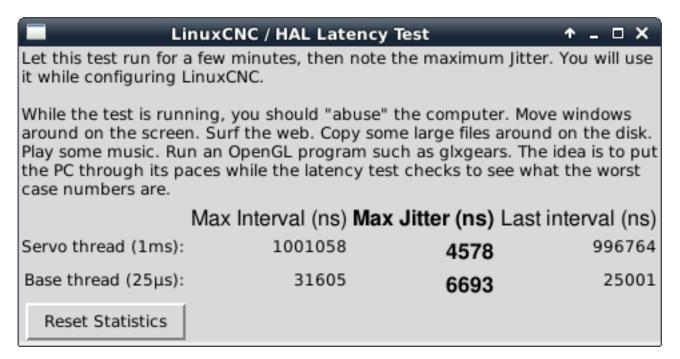
Figure 4.3: HAL Latency Test
