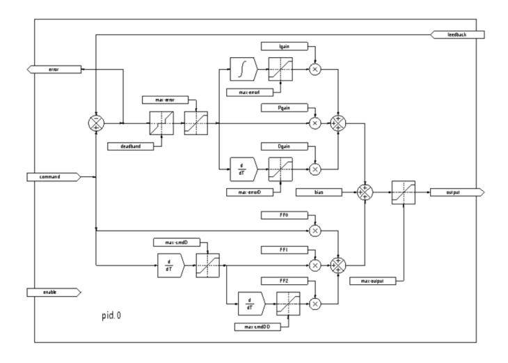
Figure 5.25: PID Loop Block Diagram
