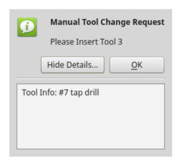
Figure 12.76: QtVCP tool\_dialog - Manual Tool Change Dialog
