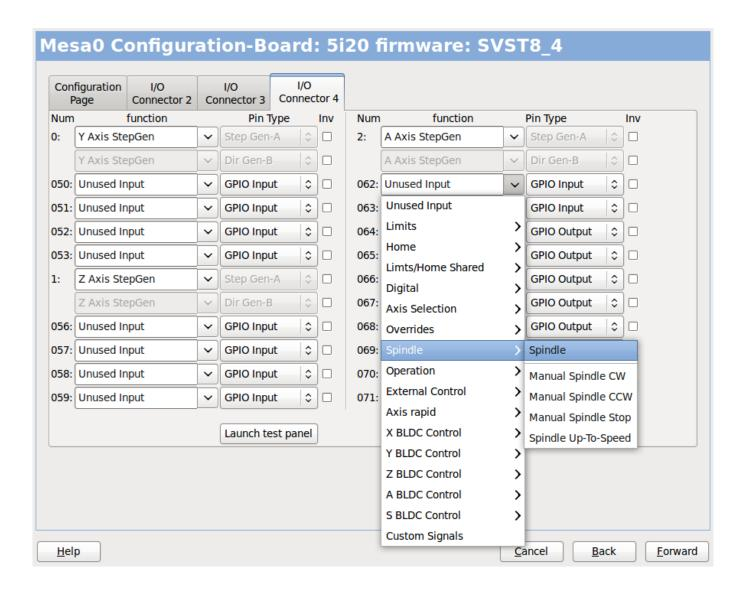
Figure 3.20: Mesa I/O C4 Setup
