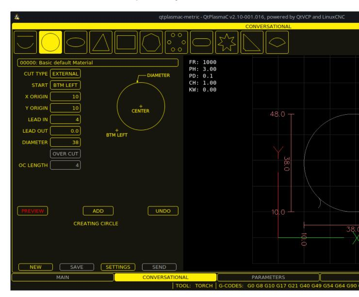
The **Conversational Shape Library** consists of several basic shapes and functions to assist the user with generating quick G-code at the machine to cut simple shapes quickly. This feature is found on the CONVERSATIONAL Tab.
