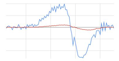
So it should be possible to compare the moving average with the dv/dt and halt THC operation once the dv/dt exceeds the normal range expected due to warpage. More work needs to be done in this area to come up with a working solution in LinuxCNC.
