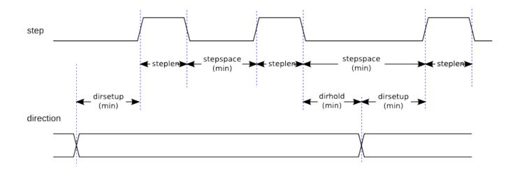
Figure 5.20: Step and Direction Timing
