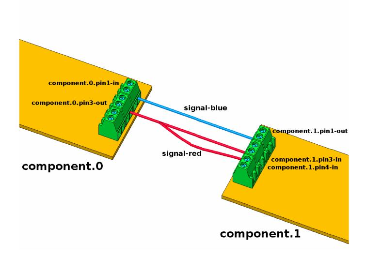
Figure 5.1: HAL Concept - Connecting like electrical circuits.
