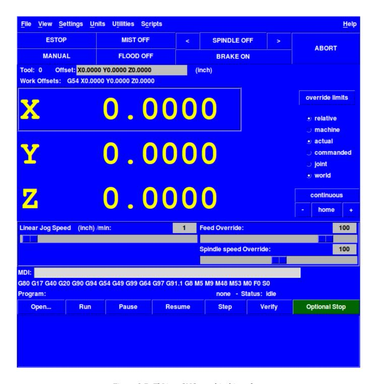
Figure 2.7: TkLinuxCNC graphical interface
