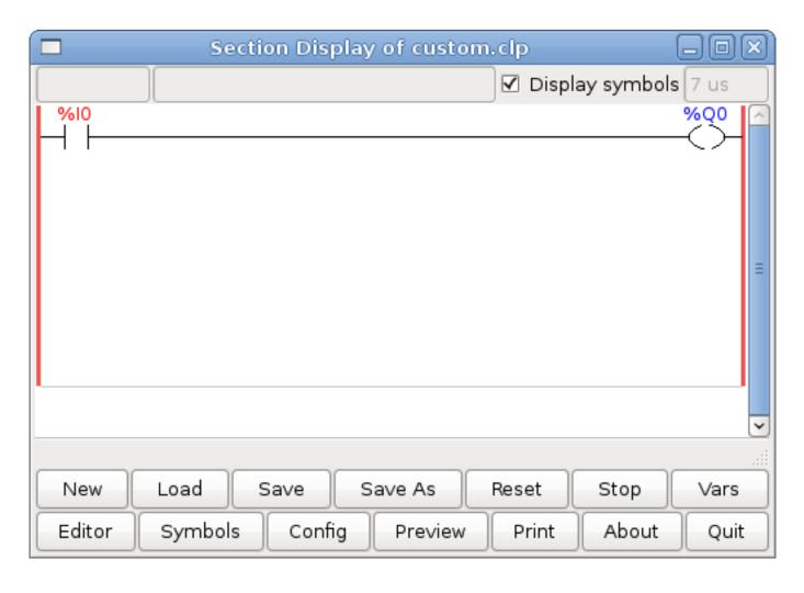
Figure 8.21: Section Display Finished
