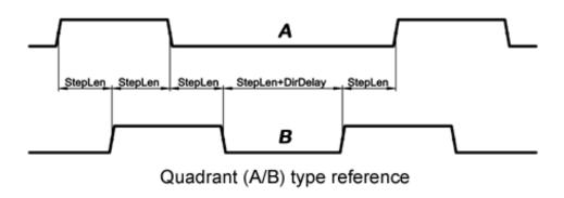
Figure 6.6: Reference signal timing diagrams
