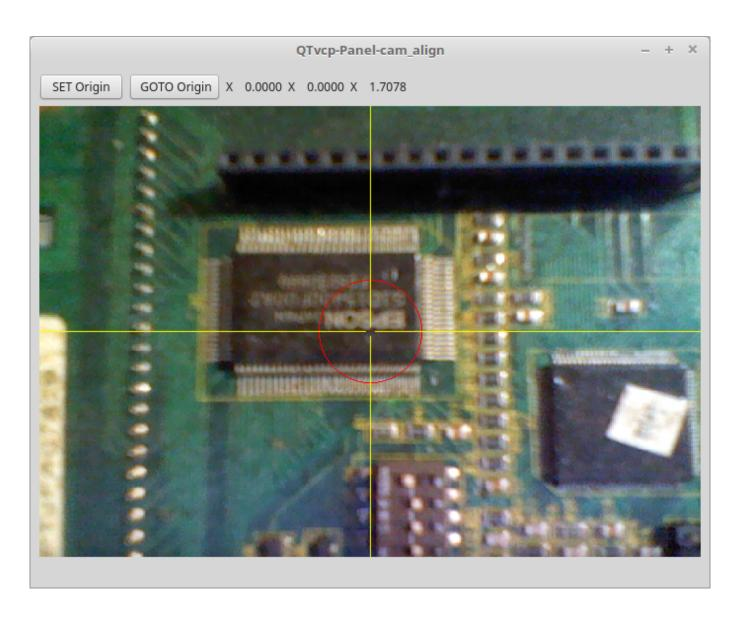
Figure 12.60: cam\_align - Camera Alignment VCP
