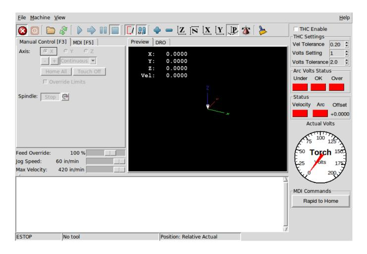
Figure 2.10: PyVCP Example Embedded Into AXIS GUI
