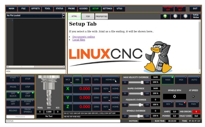
Figure 10.34: QtDragon - Setup Tab Sample
