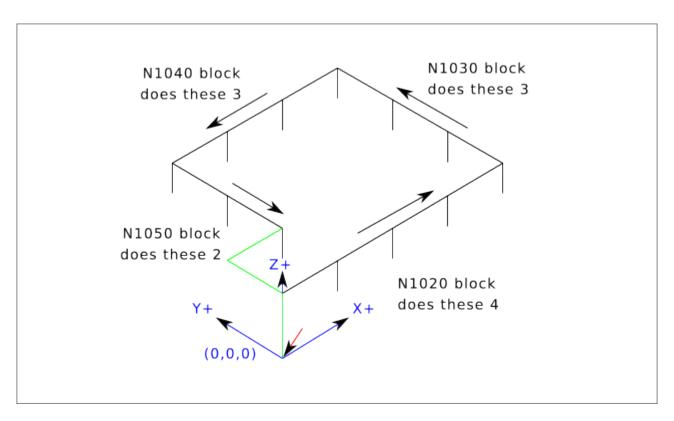
The second reason to use a canned cycle is that they all produce preliminary moves and returns that you can anticipate and control regardless of the start point of the canned cycle.
