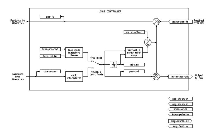
Figura 3.1: Joint Controller Block Diagram
