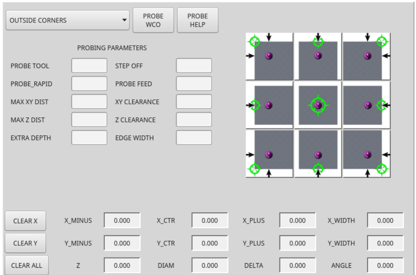
Figure 12.88: QtVCP BasicProbe: Simple Mill Probing Widget
