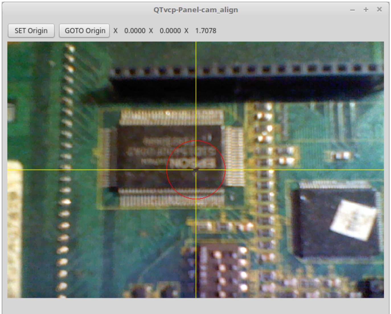
Figure 12.74: QtVCP cam_align Panel - Camera Based Alignment Panel
