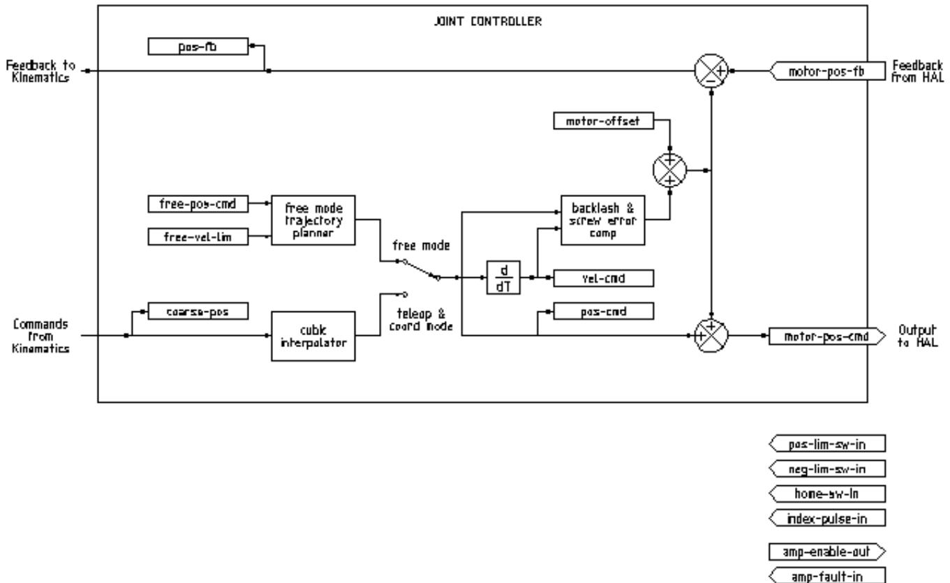
Figure 3.1: Joint Controller Block Diagram
