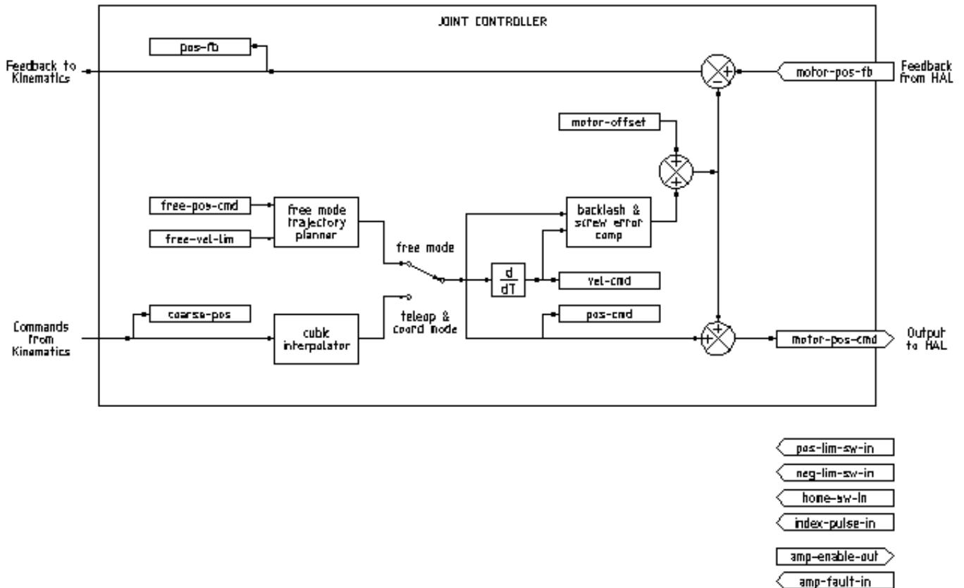
Figure 3.1: Joint Controller Block Diagram
