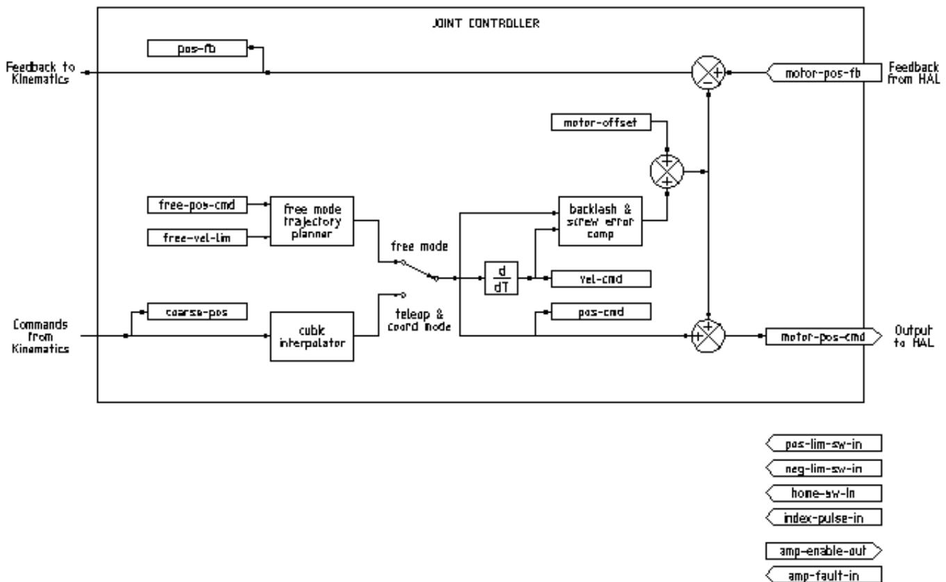
Figure 3.1 – Joint Controller Block Diagram
