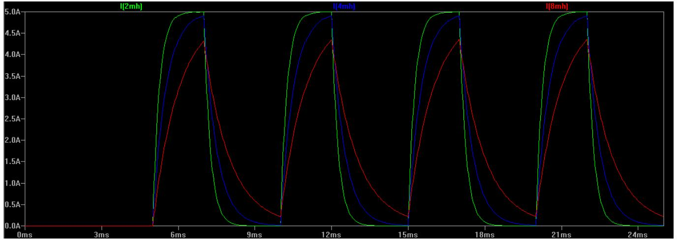
The accepted way of improving motor speed while maintaining torque is to increase the speed at which the magnetic field of the motor coils can expand and collapse. The easiest way to accomplish this is to increase the supply voltage to force the current in each winding to rise and fall much more rapidly. A quicker magnetising time equates to faster step rates while improving torque at higher speeds, both of which are obviously desirable in a CNC system.
