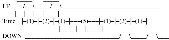
For step types 2 and higher, the exact pattern of the outputs depends on the step type (see the HAL manual for a full listing). The outputs change from one state to another at a minimum interval of **steplen**. When a direction change occurs, the minimum time between the last step in one direction and the first in the other direction is the sum of **steplen** and **dirdelay**.
