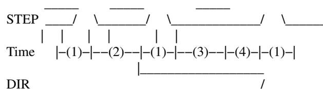
For step type 1, timing parameters 1, 2, and 5 are used. The following timing diagram shows the output
