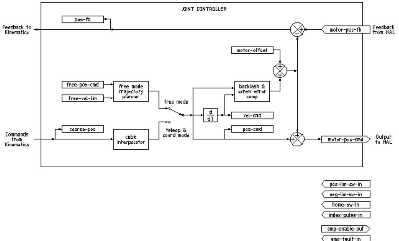
Figure 3.1 - Joint Controller Block Diagram
