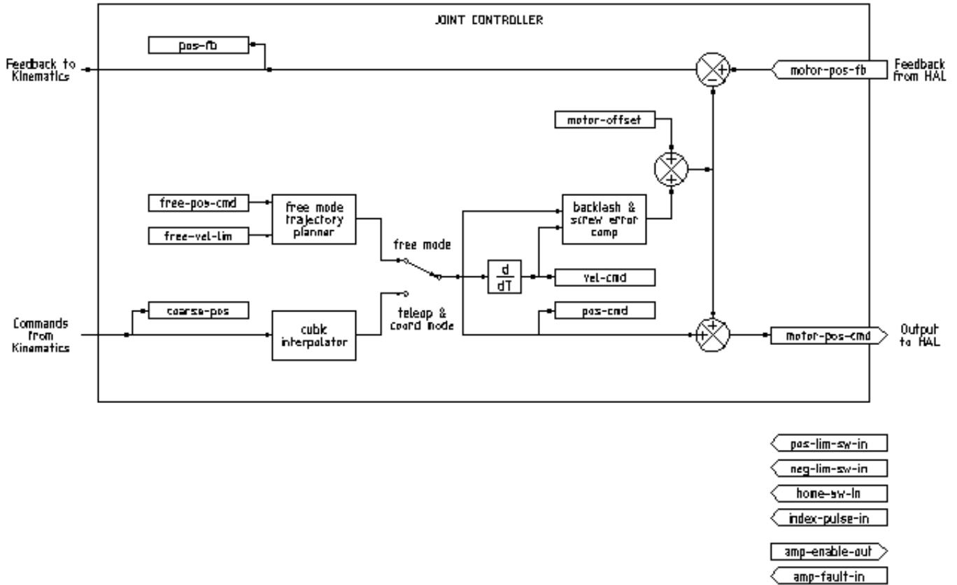
Figur 3.1: Joint Controller Block Diagram
