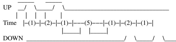
For step types 2 and higher, the exact pattern of the outputs depends on the step type (see the HAL manual for a full listing). The outputs change from one state to another at a minimum interval of **steplen**. When a direction change occurs, the minimum time between the last step in one direction and the first in the other direction is the sum of **steplen** and **dirdelay**.
