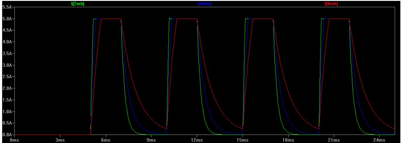
However, careful management of a higher drive voltage is required, as a higher voltage will increase current flowing in each coil with a corresponding increase in temperature of the winding. Excessive temperature rise in the winding will lead to eventual overheating and failure of the motor.
