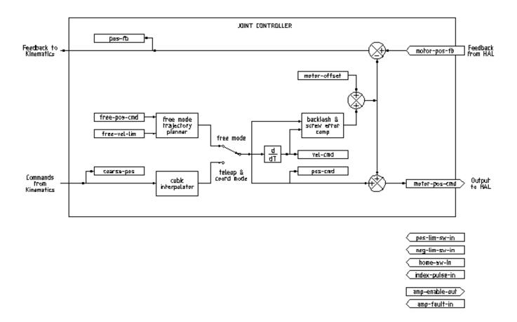
Figure 3.1 - Joint Controller Block Diagram
