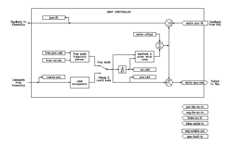
Figura 3.1: Joint Controller Block Diagram
