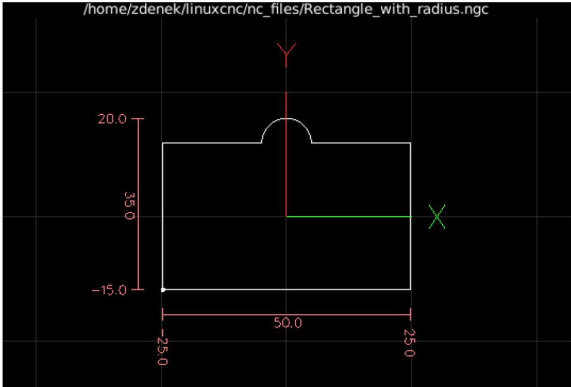
Abbildung 11.15: G64 Rectangle with radius before milling
