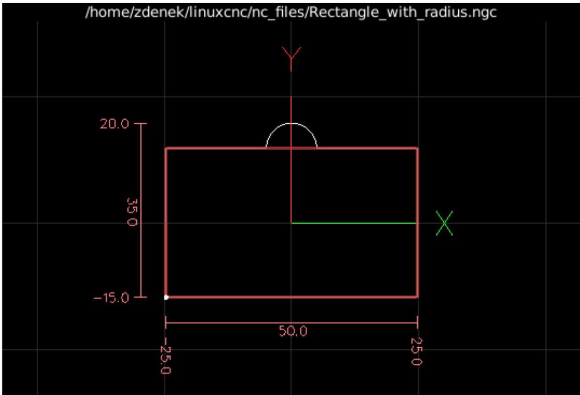
Abbildung 11.16: G64 Rectangle with radius after milling
