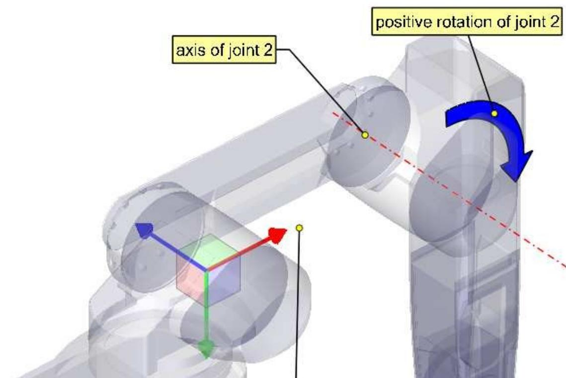
By rotating our joint-1 by  $90^\circ$  we made our X-axis intersect the axis of the next joint and we can continue defining our DH-Parameters.
