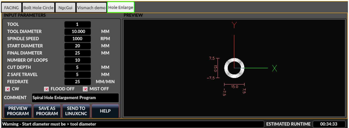
Use an end mill to enlarge a drilled hole.
